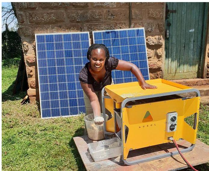
Figure 3 Solar grinding mill, Source: Agsol
